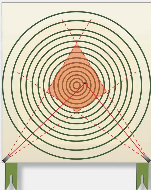
How it works: When the projectile passes through the inner target plane, it is detected completely contact- and wear free by two independent HD-infrared beams. This new technology allows for projectile detection with the outstanding accuracy of a few hundredths of a millimeter. In the outer zone of the target plane the projectile is located by five independent sound transducers. The combination of the two detection methods gives the target an outstanding cost/performance ratio.
